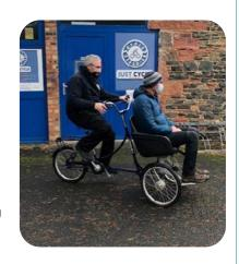
Just Cycle put a lot of work into making the bike safe, comfortable and all-terrain ready for the people we support. Workshop Manager, Grant Martin described part of the process of making the bike more accessible. "For comfort we replaced the saddle for a more padded comfortable option and fitted slightly wider tyres, along with new inner tubes to make the ride smoother over rougher ground and lessen the chances of puncturing."
